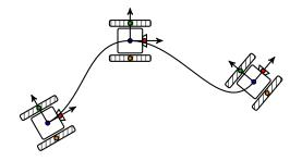
As the robot moves, we can take a snapshot of these points, and they each define a coordinate frame for Euclidean space.
