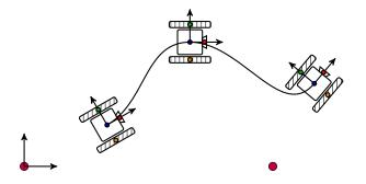
Q1: How would the robot compare observations of either purple point over time? A1: Coordinate transformations
