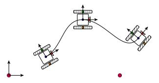
Q1: How would the robot compare observations of either purple point over time? A1: Coordinate transformationsQ2: How do we keep track of all the points on the robots?A2: Coordinate transformations, but reinterpreted. • rigid motion
