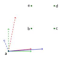
A basis and an origin together form a **coordinate frame** or **reference frame**.
