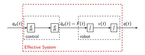
We've managed to make our robot react to desired position instantly, by
