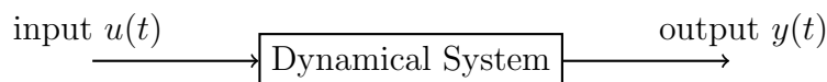
Figure 1: A dynamical system converts a function of time (input u(t) ) into another function of time (output y(t) ).
